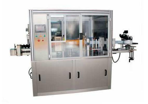
Hot melt glue labeling machine is suitable for OPP labels.
