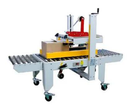
The operation process of the semi-automatic carton sealing machine: the operator adjusts the equipment according to the width and height of the carton before use. After the carton is filled with the product, the carton cover is manually closed and pushed into the machine, and then the machine automatically completes the upper and lower middle seams of the carton At the same time tape seal the box.
