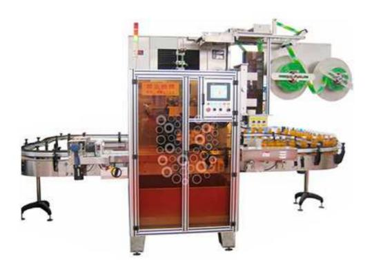
The mechanism is a kind of new-type & advanced driving device of hot shrink trapping label machine, that is, a kind of device with four-wheel drive, automatic centering and four-wheel balanced pressure, which has achieved the goals of smooth, stable and swift label transmission.
