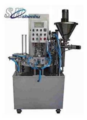
This Rotating disc filling sealing machine is suitable for the production of various kinds of products such as coffee powder. The machine made in Japan dragoness programmable logic controller, pneumatic control components, intelligent digital display temperature control system, sealed with high strength, good sealing, low failure rate, cover an area of an area small, etc, is the first choice for enterprise automation production products.
