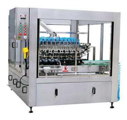
The auto glass bottle washing machine is used for washing new glass bottle before fill beverage. The washing water is clean and sterile water. The glass bottle washing machine is auto rotary type, first the glass bottle rinse turn over the glass bottle to let bottle stand upside down, and then spray the clean water into glass bottle. It is most advanced and suitable device to rinse the glass bottles. It can become a complete auto-product line, if it works with filler and sealer together.
