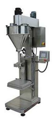
This model is designed mainly for the fine powder which easily to spout dust and high-accuracy packing requirement. Based on the feedback sign given by below weight sensor this machine do measuring two-filling and up-down work etc. It is especially suitable for filling additives carbon powder dry powder of fire extinguisher and other fine powder which needs high packing accuracy.
