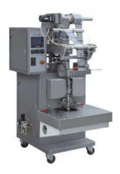
MB-280TB Series Paste-State Packaging Machine adopts Computer Control System completely; it can finish the production's process automatically such as making bags, counting, filling, sealing, cutting, printing batch number, making the rip, and so on. It also adopts the adjustable quantificational plunger pump, and it special uses for something which easy to draw bench or drip as shampoo.
