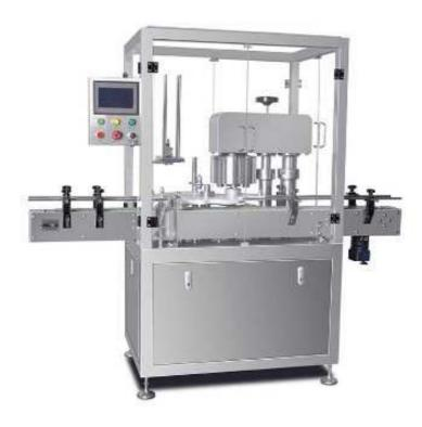
Automatic Can Seaming Machine is designed and built for seaming round tin, aluminum or composite cans. It works on the principle of rotating can. This is a standalone machine with its own conveyor belt and a fully automatic can and lid feeding system.
