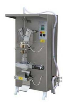
This machine is widely used in the packaging of milk, soy milk, soy sauce, vinegar, rice wine and various liquids, the entire packaging process: film sterilization, bag making, printing date, filling, sealing, cutting, counting can be completed at one time. Sealing temperature can be controlled automatically. The package is exquisite and smooth, with a stainless steel structure that meets the hygienic requirements.
