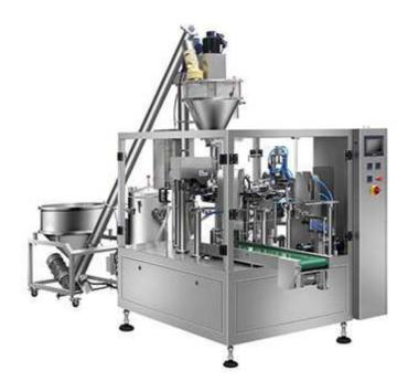
ND-BP200PO rotary packing line mainly installs rotary packing machine, screw filler and screw conveyor, suitable for packing all kinds of powder, such as milk powder, coffee, spices, additives etc...
