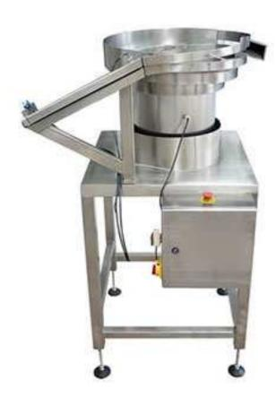
Automatic spoons feeding machine (spoons dispenser) designed to feed the spoons into metal cans or bottles before the cans go to filling station! Spoons uncrambler with vibrator which can help to queue the scoops on the feeding device before fall down to the cans.
