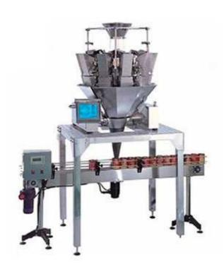
This machine is a special design for the filling of snacks dry nuts into the jars. It adopt a 10 chambers automatic electric scale which is able to dosing the nuts at extremely precise level, and the PLC and HMI control system makes it easy, direct and automatic in operating. It is your best dry nuts filling solution.
