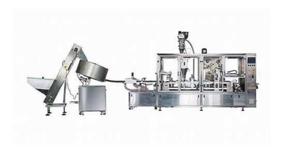
CP5004N is designed and manufactured to fit for filling ground coffee, powder into coffee capsule espresso type, upgraded speed over 50 cycles per minute.
