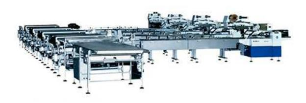
The whole Swiss roll and layer cake production line includes batter preparation system, cream preparation system, jam preparation system, forming roller, oven tunnel, bench conveyor, sliter, alcohol depositor, cream/jam extruder, layer cake forming equipment, ultrasonic cutter, turn conveyor, chocolate decorator, cooling tunnel and packing line.
