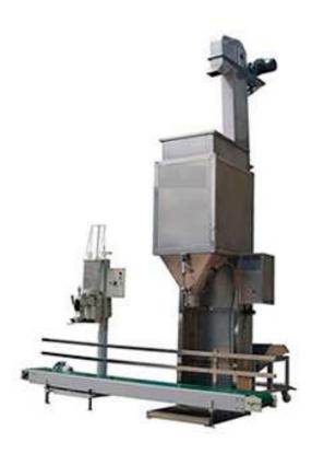
The LCS small single bucket weighing and packaging machine is a quantitative bagging device controlled by a computer, combining mechanical feeding and electronic weighing. This machine has the characteristics of accurate measurement, intuitive display, simple operation, reliable performance, low noise, stainless steel and corrosion resistance, etc. It is an ideal small quantitative packaging equipment.
