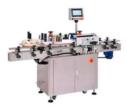
KL-700 main parts would be labeling head, stainless steel 304 frame, conveyor system, sponge pressing while and Siemens PLC touch screen and servo motor for fast speed labeling.
