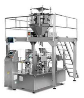
This automatic doypack machine system consist of 8 stations rotary packing machine, 14 heads combination weigher, Z shape bucket elevator and platform. With SIEMENS PLC and HMI, FUJI frequency converter, the machine can works at a maximum packing speed 60 bags per minute.
