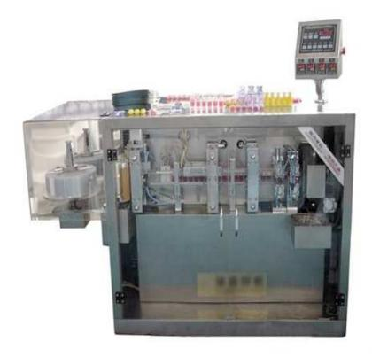
DG-118 Oral Liquid Plastic Bottle Filling and Sealing Machine is group molding machine for plastic containers from material of PVC and PE, and filling them with the subsequent sealing. It's unique model without analogue in the world market.
