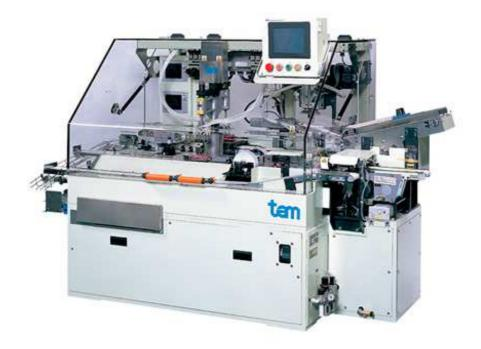
The CN1000 automatically fills and pack elongated product items such as stick-packed gum or candy. It improves your production efficiency even further when this cartoner is included as part of your production line. The products are filled into carton by swiveling pick and placing device and operation output of 200 pcs per minute can be achieved.
