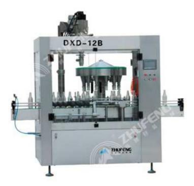
This machine adopts PLC program control, rotary in and out of bottle, dial positioning. Photoelectric detection for bottle, if have no bottle and will not to filling. Screw discharge measurement, the speed of producing is high. It is suitable for all kinds of particulate and microparticles powder filling.
