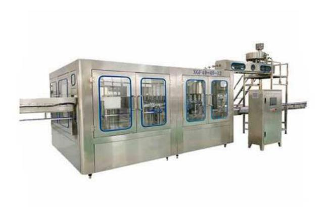
This automatic mineral water filling machine mainly used in the water filling operations, the three function of bottle washing, filling and capping are composed in one body of the machine, the whole process is automatic, it is conveniently trunked to adjust the machine to fill various types of bottles, the filling operation is faster and more stable due to the advanced filling valve technology, The famous brand programed controller (PLC) is adopted to control the machine runs automatically.
