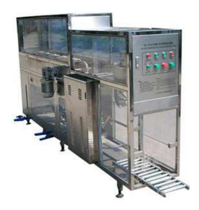
It included 4psc washing station: city water washing & pure water washing. 1psc filling head statiopn, 1psc pressure capping station. It is the most cheap 5gallon business machine. One machine produce 5gallon bottle water can for one town people inquiry.
