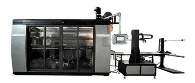
The whole Plastic Cup Thermoforming Machine Mainly for the production of variety plastic containers (jelly cups, drink cups, disposable cup, package containers, food bowl etc) with thermoplastic sheets, such as PP, PET, PS, PLA, etc.
