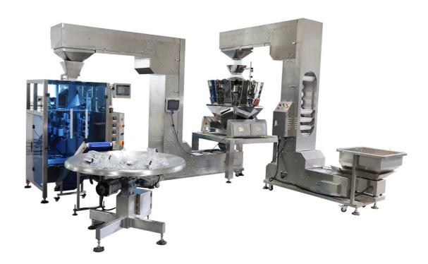
The automatic celling height limit combination packaging solution is suitable for limited height space, but must go with multihead weigher packing machine; this is will be the best solution which twice feeding system, and the second feeder can be changed into Z type material elevator accordingly with same function; the dimple multihead weigher is for different foods package.
