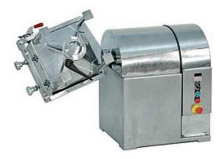
**PMS Container Mixer®**, which is normally known as intermediate bulk container (IBC) mixing system, is a mixing system that is widely used within pharmaceutical manufacturing process. This type of mixer can be used as storage, transport, and mixing vessel, which reduces the complication of the conventional mixing processes that require a number of containers for the whole process.
