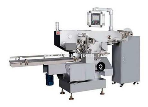
SL-SBGB450 series packing machine is designed for rectangle chocolate confection and folded on the side. It is widely used in chocolate and candy packing. And also apply to other fields (with proper hardness but fragile or not easily handled), such as Arabic spice stick, etc. With the advantage of fast packaging, good consistency, low failure rate, and long service life.
