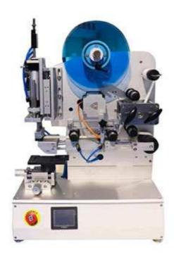
It is suitable for labeling on the upper plane, curved surface and concave surface of the product with a labeling accuracy up to 0.2mm. It is mainly used for precision labeling of electronic components and digital products, such as SD card, mobile phone battery, FPC and mobile phone charger. High precision labeling, highlighting the excellent quality of products, improve competitiveness.
