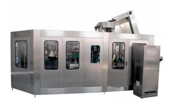
BGF16-12-6 This type of glass beer bottle filling machine is specially used for equal pressure glass beer filling. Filling adopts suction technology, which has the function of automatically closing the bottle valve and flushing broken glass, and shock with hot water before opening the stopper.
