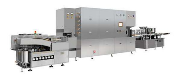
The oral liquid washing-drying-filling-capping production line is composed of the QCL series vertical ultrasonic bottle washing machine, ASMR tunnel hot air circulation sterilizing oven and YGZ series oral liquid filling-capping machine. Suitable for production of oral liquid bottles of 2-25ml, it can complete such procedures as water spray, ultrasonic washing, water filling, gas charging, drying, sterilizing, cooling, filling, capping, and etc.
