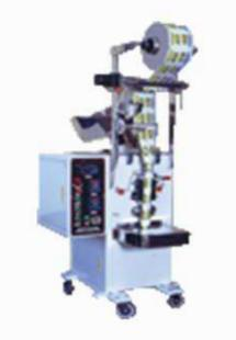
This series of machines are suitable for packing of pillow-shaped of tablet. Automatically accomplish packing, making sack, filling, cutting, sealing and counting.
