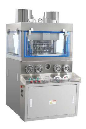
This machine is an automatic double pressure rotary tablet press, which can press grains into round, engraved texts, special shapes and two-color plate recipes. Mainly used for the manufacture of prescription tablets in the chemical, food, electronics and other pharmaceutical industries. (Note: When producing two-color sheets, simply replace the components and add a powder suction device, which will greatly reduce costs and increase profits.)
