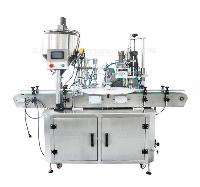
This automatic packaging machine is designed with multiple function; it can fill liquid or paste, feed bottle caps and cap bottles automatically. The multifunctional filling and capping machine can help you save production cost and space. This machine is suitable for essential oil, water, juice etc. This machine is suitable for filling different sizes of containers at the same time.
