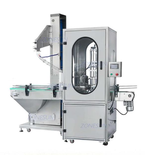
Designed for F-style bottles, this automatic capping machine is with function of feeding bottle caps, and the working height can be adjusted according to bottles. It is widely used in chemical industries.
