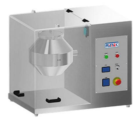
Double Cone Blender operates on the free flow principle. This unit is used for dry blending, rapid mixing of all types of free-flowing powder and granules, mixing, lubrication and homogenizing of the powder and granules. It consists of a cone-shaped body, a circular central portion and top and bottom conical. The uniform, multidimensional arrangement of the Blender walls ensures good blending and mixing. The vessel is manufactured from stainless steel.
