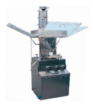
An economical automatic continuous rotary high-speed tablet press, the series ZP1100 A rotary tablet press is mainly used in the tablet production in pharmaceutical factories. The machine is also applicable to foodstuff, electric cell, chemical and electronic industries to press the granular material into tablets.
