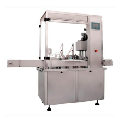
This machine is able to finish procedures automatically as converting, filling, corking, capping, with sending caps structure of oscillation bucket, corking and capping with air press.
