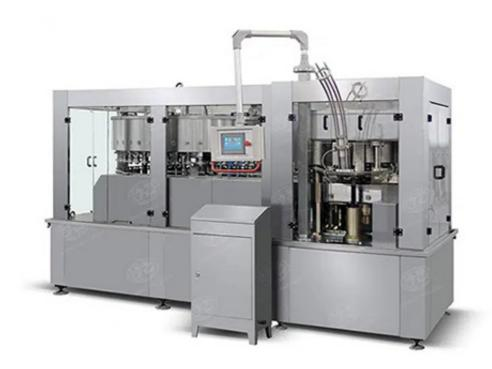
The can beer filling machine is special designed for medium capacity brewery. The can beer filling line has easy operating with high efficiency. The working flow includes CO2 purge, filling and then sealing the caps.
