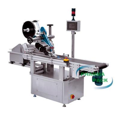
Designed for labelling flat bottles at a speed of up to 200 bottles per minute. Label dispenser adopts servo motor to drive; dispensing label implements closed-loop control; label dispensing accuracy can be 0.2mm; max. label dispensing speed is 60 meters/min. With the storing parameter function, labeler can store about 50 groups of parameter information, to be adjust them conveniently, can reduce time to debug machine when labeler is adopted to product many kinds of products.
