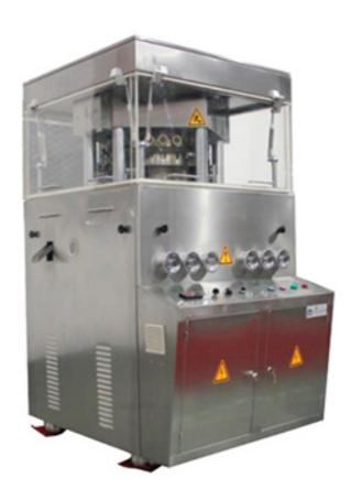
This machine is used to press all sorts of granular materials, like geometry shape of profiled sheet, double lettering piece, traditional Chinese medicine tablet, western
