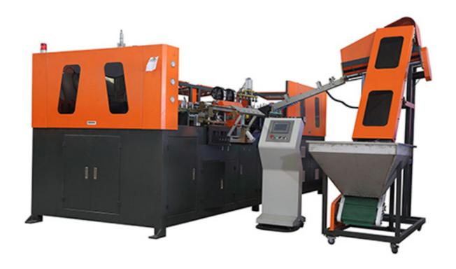
Full-automatic PET bottle blow molding machine is the most stable two-step automatic stretch blow moulding machine. PET bottle blowing machine has two cavities to six cavities and the maximum volume of the products is 2000ml. The speed is 1000 bottles per hour per cavity (based on 500ml bottle).
