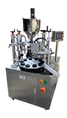
The process of tube sealing machine eliminates the use of glue and allows the thermoplastic parts to bond to itself. Ultrasonic sealing with the proper time setting and pressure is the fastest most reliable method for a variety of tube material sealing.
