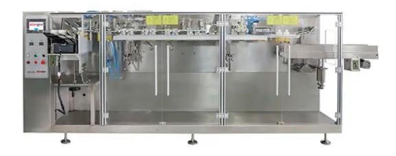
BHP-240 is specially designed for medium-sized bags. It can pack a variety of bags. It is easy to change bag types and sizes. It has a wide range of applications. It can pack liquids, solids, granules, powders, viscosity, etc., reducing bag making functions and improving packaging speed and efficiency.
