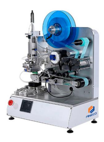
FK618 is suitable for all kinds of specifications square, flat, tiny curved and irregular products high precision and high overlap labeling, such as electronic chip, plastic cover, cosmetic flat bottler, toy cover.
