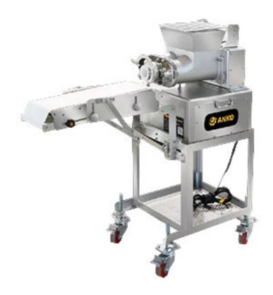
How to produce icebox cookies quickly? To make slices of icebox cookies, the dough should be shaped and refrigerated until firm before slicing it into a perfect shape. For mass-producing, it consumes time and energy to shape every dough by hand. Now, by putting cookie dough into the dough hopper, the machine can extrude the dough into a shaped bar for the sequential refrigerating and slicing processes.
