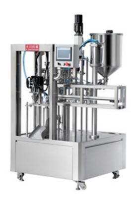
The DC-230/DC-230S is suitable for filling and capping chilled food products such as yogurt, soy milk, soy yogurt, and juice in self-standing pouches. The product features accurate filling, thorough cleaning, tight capping, and reliable quality. The machine will not fill without a pouch and will not cap without a lid; electromagnetic capping (servo motor capping is optional).
