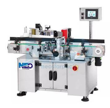
Automatic round bottles labeling machine LR4000 is available for any kind of erective plastic bottle and glasses labeling such as water bottle, yoghurt, wine bottle, seasoning, cleanser, small round bottle, ampoule, nail polish, lipstick, mascara, lip gloss, battery etc. Different kind of label like transparent label, anti-forgery label and barcode label are all applicable to this machine.
