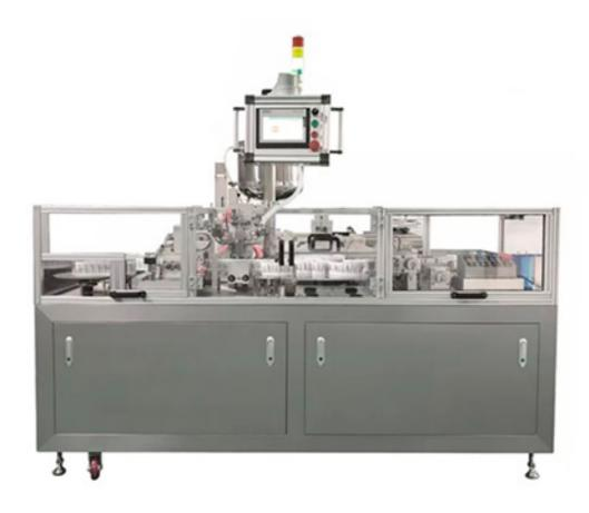
GSJ-1B suppository filling production line has stable and efficient filling, sealing and other production processes, and production capacity of 1000-1500 pills per hour. Semi-automatic suppository filling machine differs from a fully automatic suppository production line in that the latter includes a suppository bottle forming function.
