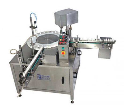
Laxmi Pharma Equipment introduces Automatic/Semi-Automatic Rotary Type Plastic Vial Eye Drop Filling & Sealing Machine Mode series': LRVFS.
