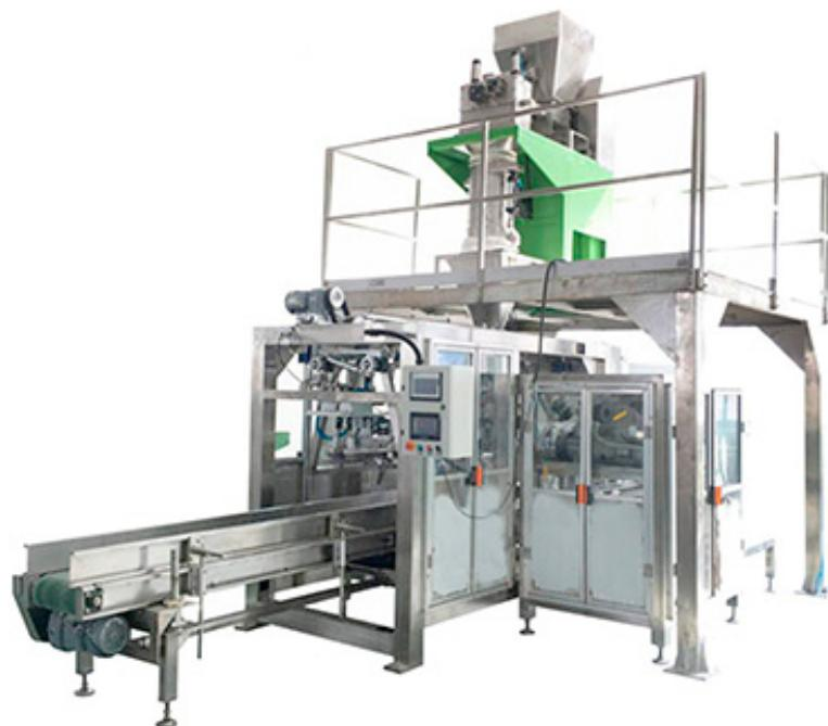
ZLCP-50P Automatic powder bag feeding packaging machine unit is specially suitable for powdery material, the packaging material is paper bag, PE bag, woven bag, the packing range is 10-50kg, the maximum speed can reach 3-8 bags/min. High efficiency, advanced design suitable for various requirements.
