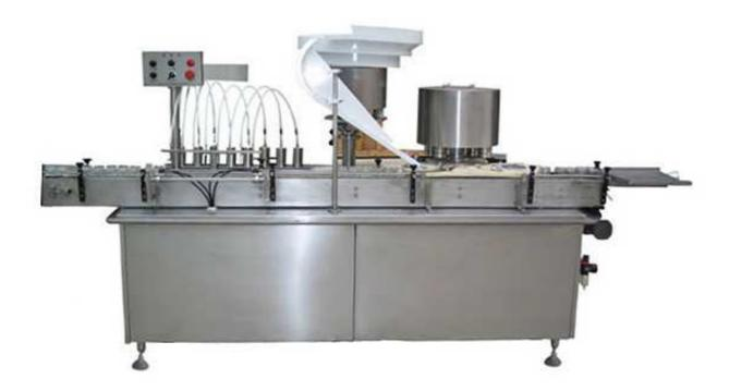
This machine is the main filling equipment of the liquid filling production line, which is mainly applied in the filling and sealing of 30 – 500 ml glass bottle or plastic bottle. Automatic feeding, 8 to 12 filling nozzles, 4 screw cap( or cover rolling), send to cover electromagnetic vibration.
